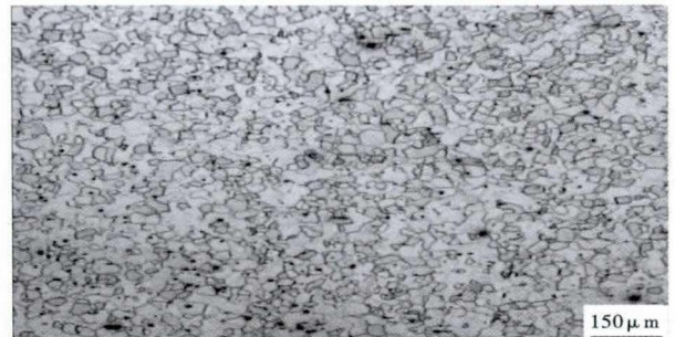
图 3 HC250IF 钢带组织形貌 Fig. 3 Morphology of structure of steel HC250IF strip
