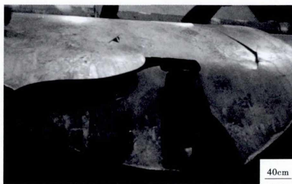
图1 4.3 mm热轧带钢HC250IF拉矫断带形貌 Fig.1 Morphology of 4.3 mm hot rolled strip fracture during straightening process of steel HC250IF
